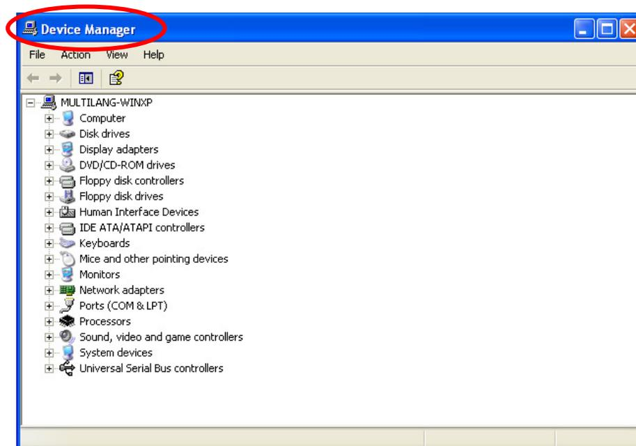
3. Click the "+" by "Ports (COM & LPT)". You should see the Prolific USB-to-Serial Comm Port (COM3) device listing. This also means that Windows has assigned the device to COM3 port..
