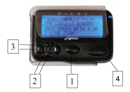
•TO PROGRAM PAGERS, REMOVE BATTERY AND HOLD DOWN BUTTON 1. INSERT BATTERY AND HOLD BUTTON DOWN UNTIL PASS CODE SHOWS IN THE DISPLAY PRESS BUTTON 4 TO CHANGE TO FREQUNCY SCREEN
